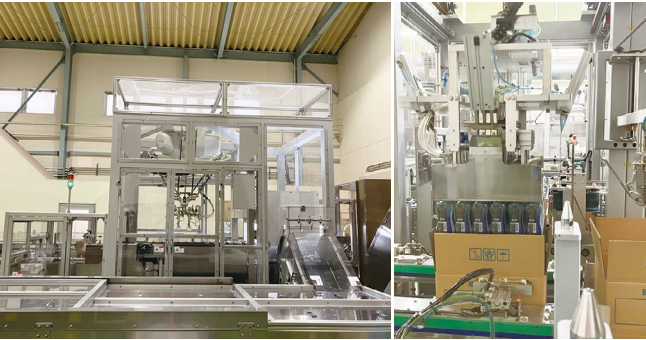
Kashima Oil Filling Plant: An industrial robot that keeps empty bottles in line and places them into a box
