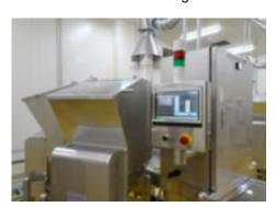
Automatic weighing instrument
